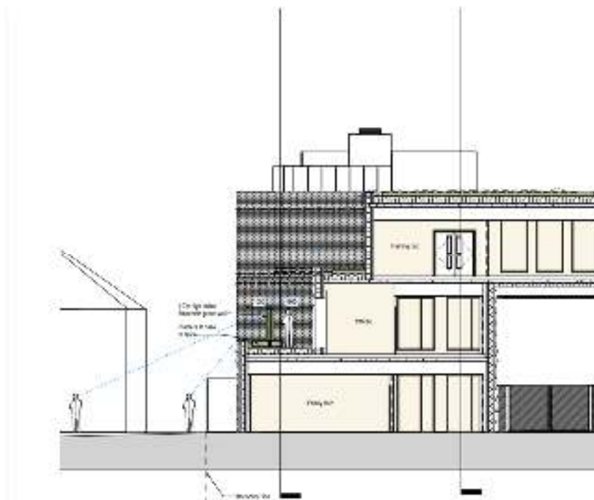
Fig 4a – section showing enclosure of terrace
